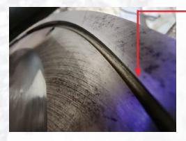
When a Flywheel has a relief (dust ring) at the transition from the friction surface to the clutch pilot ring, the relief must remain after resurfacing or your plate will not sit flat against the flywheel. If your flywheel has been resurfaced multiple times or the wear was significant enough to result in this relief being machined out during resurfacing, you NEED a new flywheel.
