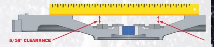
The clutch pilot ring should be no more than 3/16 tall as measured from the machined friction surface to the top of the pilot ring.
